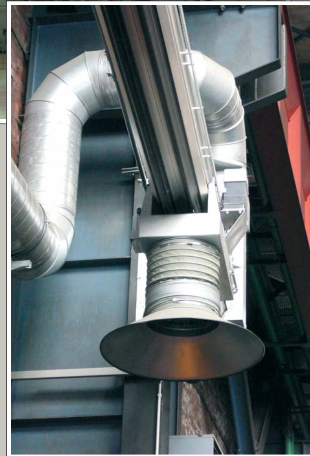
Rail system SSK 900 with swivel extractor arm and inside movable telescope exhaust nozzle diameter 450 mm for 10,000 m 3 /h with electrical drive for all three coordinates. Optional radio remote control.
