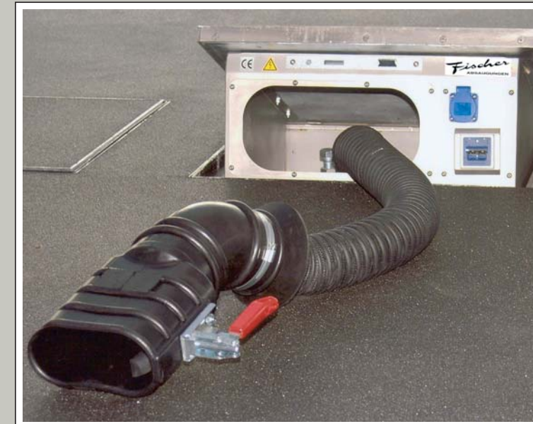
Underfloor extraction system with pull-out exhaust gas hose, rotatable bended nozzle 60° and gripper nozzle with clamping pliers for dual-pipe exhaust systems incl. power supply, pneumatic operation. The system is delivered as a complete fitted component with high temperature tubing for stub lines and connected to a central fan type FD.
