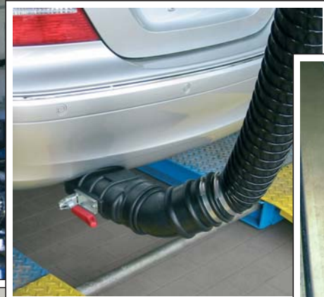
Exhaust bended nozzle 60° with swivel coupling and attached dual pipe nozzle with clamping pliers.
